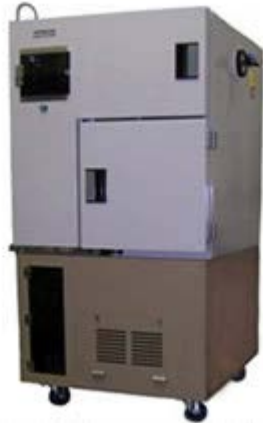
Fig.1. Prototype completely closed compact automatic cell culturing equipment (volume 900ℓ, floor space 0.6m 2 )
