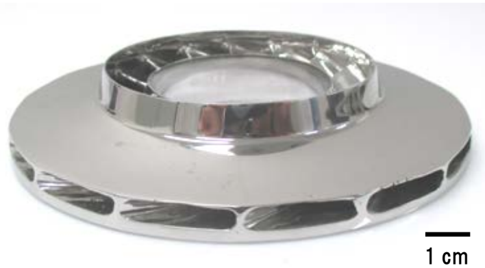
Figure 2: Impeller with complicated shapes successfully formed by test molding
