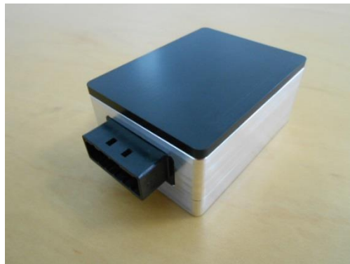
The newly developed 77GHz millimeter-wave radar (30 mm in depth, 60 mm in height and 45 mm in width)
