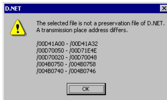
Figure 4-113 Error Message Dialog Box Reporting on an Invalid D.NET Setup Info File Specified
