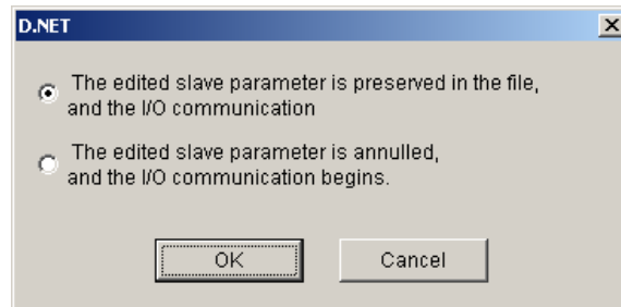
Figure 4-52 A Confirmation Dialog to Confirm Whether or Not You Are Saving the Slave Parameter Setting File
