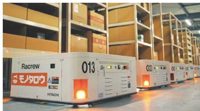
Racrew, a compact and low-floor automated guided robot in operation at the MonotaRO Kasama Distribution Center
