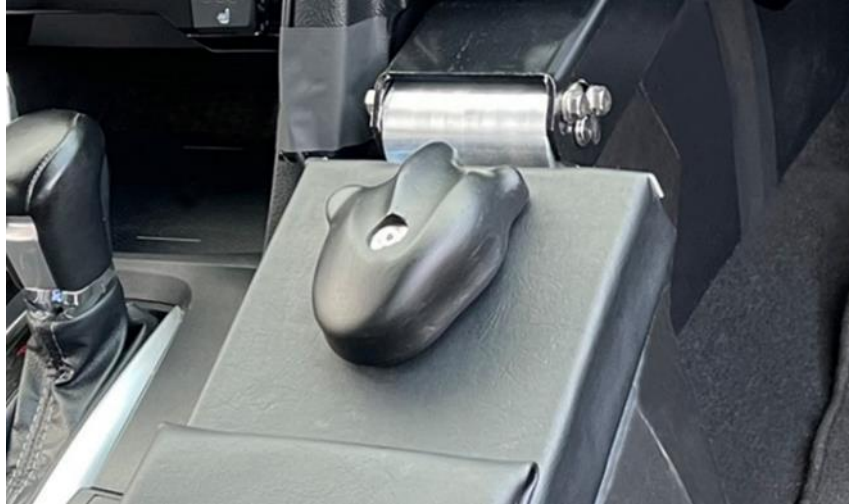
Prototype of new steering device that expands the cabin space
