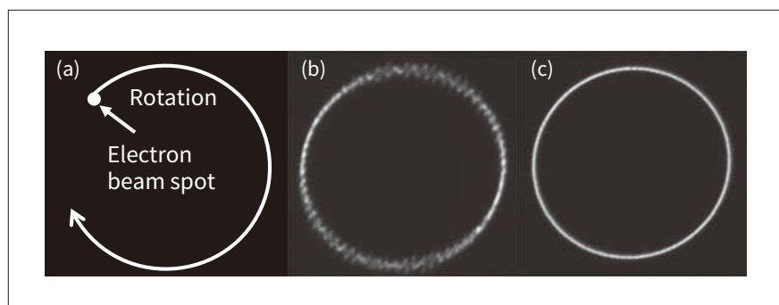
**Figure 2—Explanatory Diagram of Test to Visualize Beam Fluctuation and Example of Test Results Before and After Noise Elimination Measures**
