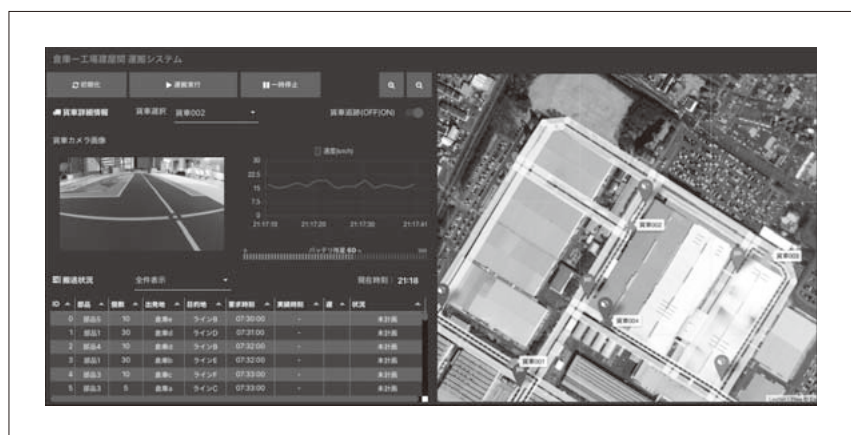
Figure 2 — Dashboard Screen Created Using Node-RED
