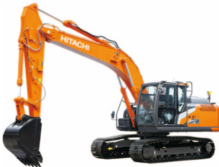
1 ZX200X-7 ICT hydraulic excavator
