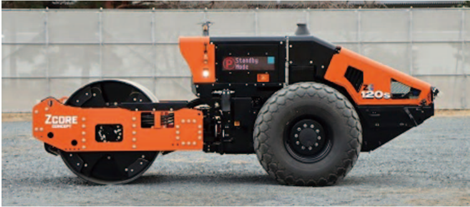
5 Autonomous compaction system unit
