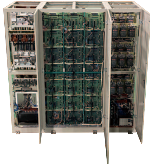
1 New 350-kW multiport EV charging system
