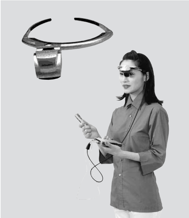
Fig. 2—The External Appearance of the HMD and How It Is Worn.
