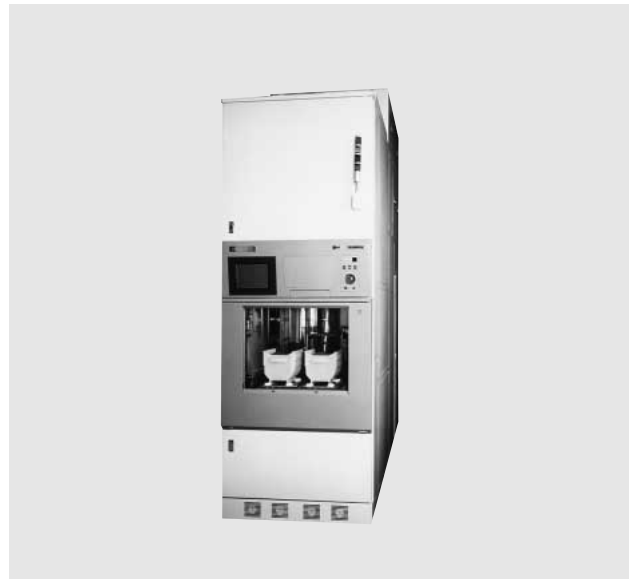
Fig. 1 — SiGe Epitaxial Growth System VERTRON-V (SE). The ultra-clean low-pressure CVD system for batch SiGe epitaxial growth, proposed by Hitachi Kokusai Electric Inc.
