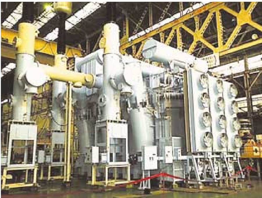
Fig. 1—View of Shop Test of 281.25-kV (525-kV) 1,060-MVA Double Rating Voltage Transformer. The shop test would be carried out by using test bushings, although the secondary side was connected with power cable. The test was first carried out in the 525-kV connection state and was repeated after changing to the 281.25-kV connection.
