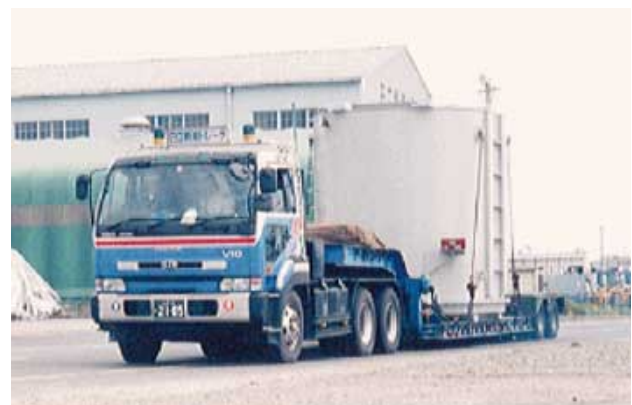
Fig. 5—Transportation Test. An electrical characteristic test was carried out before and after the transportation test.
