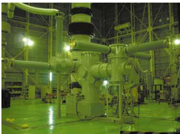
Fig. 6—Withstand Voltage Test on GIS. The test confirmed withstand voltage performance at all parts as specified.
