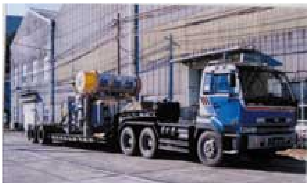
Fig. 5—Transport of GIS. Transportation tests demonstrated that one fully assembled bay could be transported without any problem.
