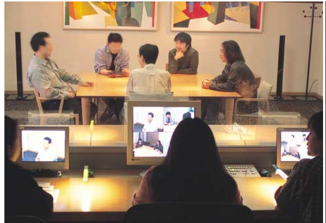
The usability laboratory “FACE,” which allows observation of the users activity through the one-way mirror.
