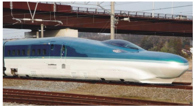
Fig. 2—High-speed Test Vehicle of Type E955 Shinkansen “FASTECH360Z” (train for new and existing direct routes). Type E955 is the Shinkansen for tying together new lines and existing lines (without the need for train transfers) aiming at a 360-km/h commercial service.
