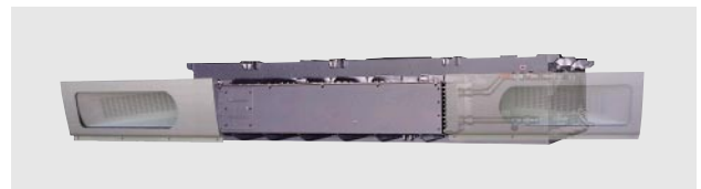
Fig. 3—External Appearance of the Main Converter of the Water-cooling System Utilizing Air-flow during Train Running. By fitting a water-cycle-cooling system using airflow generated during train running (thereby eliminating the need for electrical air circulation), a compact, lightweight, and low-noise main converter was accomplished.
