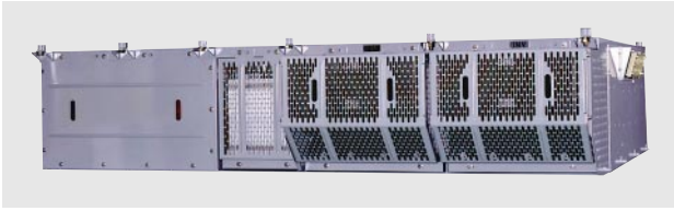
Fig. 3—Main Converter. The inverter equipment, converter equipment, and SIV (static inverter) are combined, thereby achieving compactness and weight-saving.
