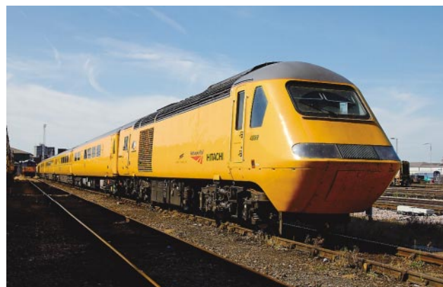
Fig. 6—Test train “V-train 2.” The test train—fitted with the hybrid system—has undergone repeated running tests incorporated into the existing railway structure in the UK.
