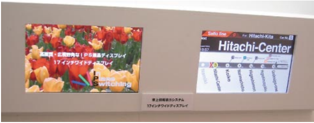
Fig. 6—IPS LCD Panels Fitted above Opening Doors for Imaging Current Interior Situation. By providing high-resolution images, added value is increased.
