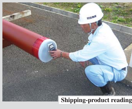
Fig. 3—Examples of Scenes of Workers Using RFID Technology and a Work Input Screen at Pipe-production Plant. RFID technology is applied to work-record collection and welding control as well as shipment control of piping.
