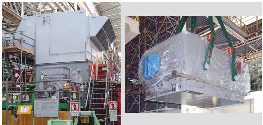
Fig. 1—Shop Test (Left) and Transfer by Indoor Crane for Delivery (Right) of GH1550A. The GH1550A air-cooled generator underwent various tests including rotational tests in the factory, and in doing so its performance and design were validated.
