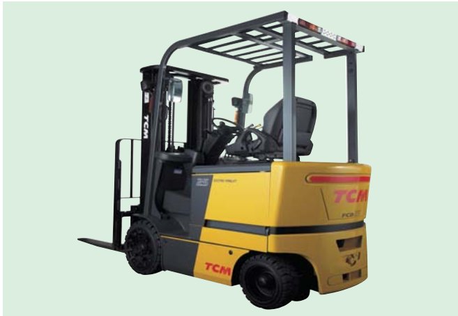
Battery forklift with cushion tires (maximum load of 2,500 kg)
