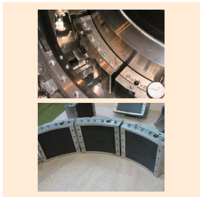
Bearing assembly (upper) and bearing surface (PPS) (lower)
