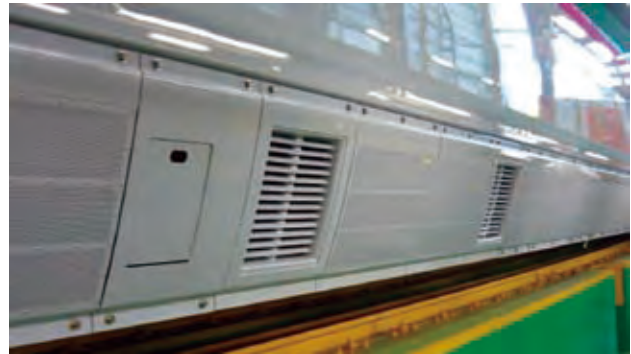
Fig. 2—Side Cover with Sound Absorbing Material on E5 Series Shinkansen (Prototype Model).
