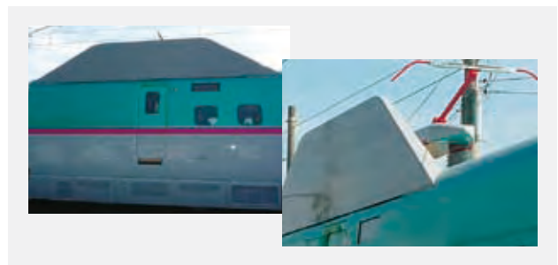
Fig. 3—Pantograph and Noise Reduction Plate on E5 Series Shinkansen (Prototype Model).
