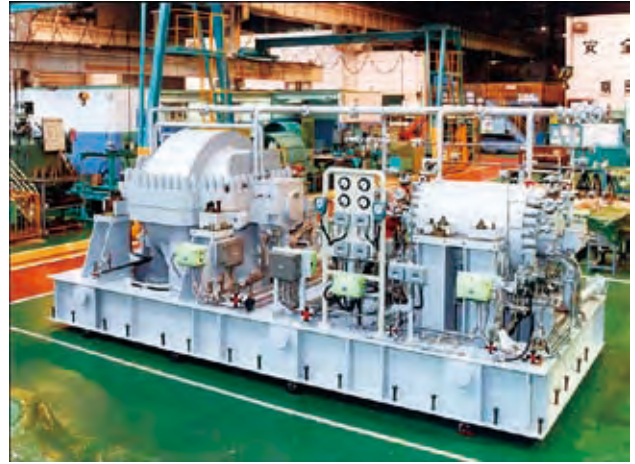
Fig. 7—Centrifugal Compressor for CO 2 Liquefaction. A centrifugal compressor for liquefying CO 2 delivered to a urea synthesis plant in China is shown. The unit is powered by an 8,200-kW steam turbine and uses two casings to compress CO 2 gas from atmospheric pressure to 18.3 MPa.
