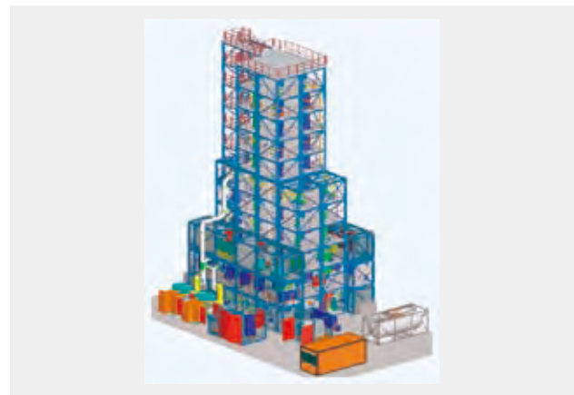
Fig. 6—Outline of 5,000-m 3 N/h Mobile Pilot Plant. The outline of a pilot plant designed to conduct testing using actual flue gas in Europe is shown. Evaluation trials at existing power plants are planned to start from mid-2010 as part of joint research with a German utility companies.
