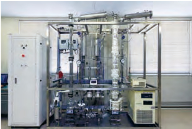
Fig. 3—Bench-scale Test Apparatus. The properties of solvents suitable for the flue gas of coal-fired boilers were evaluated using a gas that simulated flue gas.
