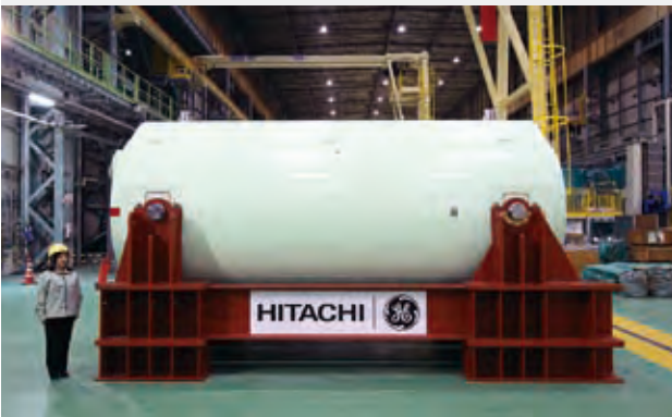
Fig. 2—Recyclable-Fuel Storage Center and Actual-size Cask. The Recyclable-Fuel Storage Center to be constructed in Mutsu City in Aomori Prefecture (top) (photograph courtesy of Recyclable-Fuel Storage Company) and a metal storage cask produced by Hitachi (bottom).
