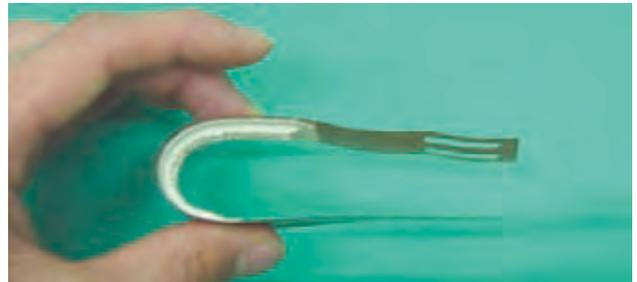
Fig. 7—Flexible Eddy Current Testing Probe. The flexible eddy current testing probe can be bent to follow curved surfaces as shown here.
