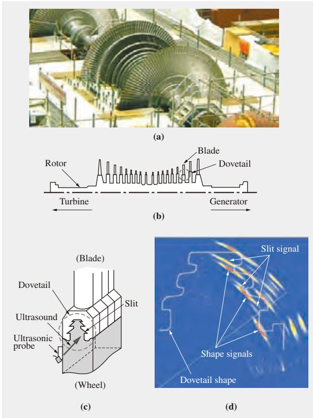
Fig. 2—Ultrasonic Testing of Dovetail Joints in the Low-pressure Rotor Wheel of a Steam Turbine. Steam turbine (a), axial cross-section of steam turbine rotor (b), dovetail joint and probe position (c), and image of dovetail joint captured by phased array ultrasonic testing (d) are shown.
