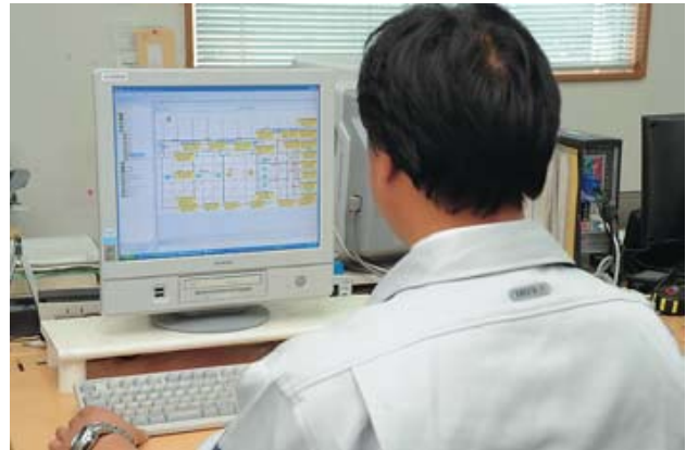
Fig. 4—Sensor Network Information System in Use. Hitachi's sensor network management software allows users to review all of the temperature and humidity data from the warehouse from an office PC (personal computer).
