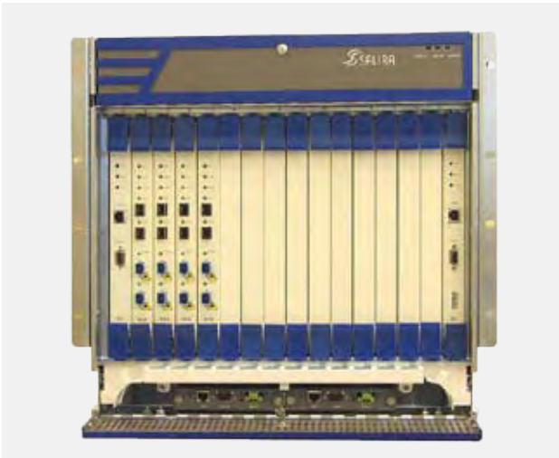
Fig. 5—DePON OLT. The OLT consists of PON interface terminators and a monitoring and control interface.
