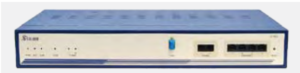
Fig. 6—DePON ONU. The ONU provides the end user with triple-play services and a wireless LAN (local area network) access point.
