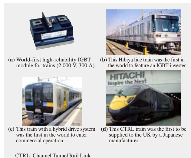
Fig. 7—World-first IGBT Module for Trains and Example Trains Fitted with IGBTs.
