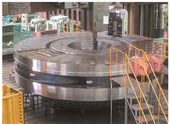
Splitter-blade pump-turbine runner under construction for Okutataragi Power Station of The Kansai Electric Power Co., Inc.
