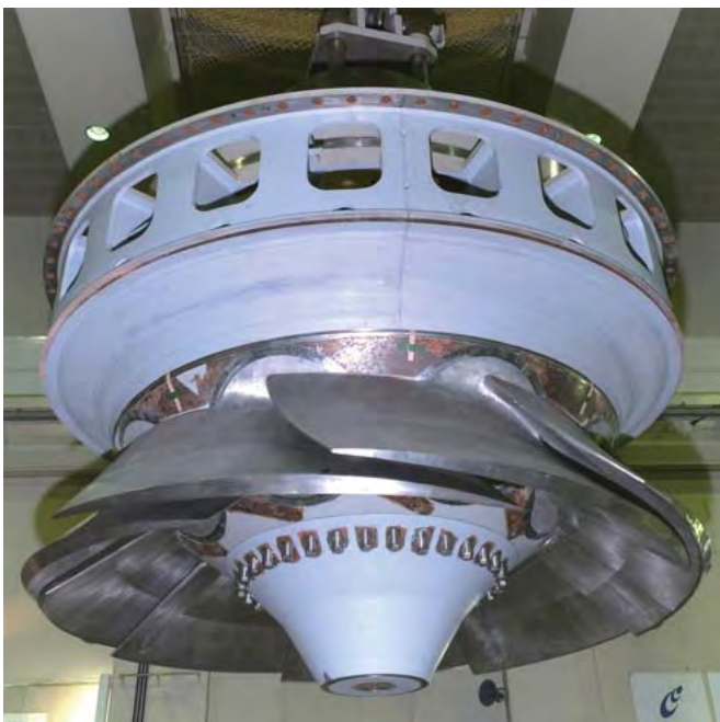
Photo of a rotating servo motor being reassembled in the factory after refurbishment
