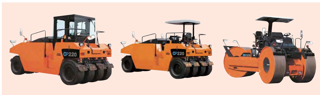
From the left, the ROPS cab tired roller, standard canopy tired roller, and standard canopy macadam roller
