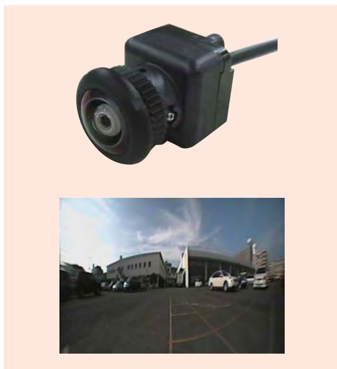
Ultra-wide-angle vehicle-mounted camera (top) and example screen (bottom)
