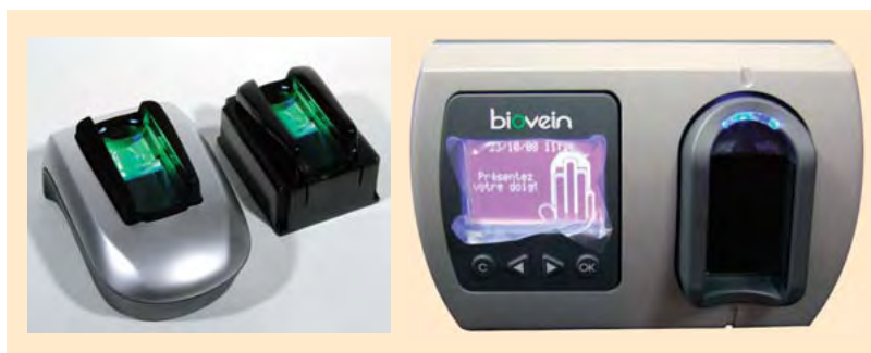
First multi-modal device (fingerprint and finger vein) (left) and finger vein-based physical access control system (right)
