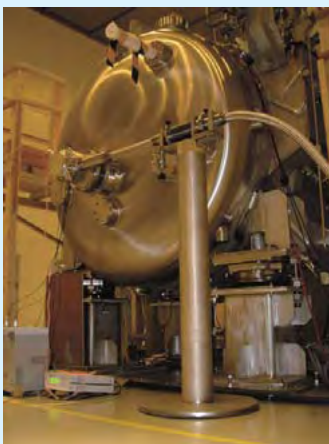
Split superconducting magnet for new NMR method
