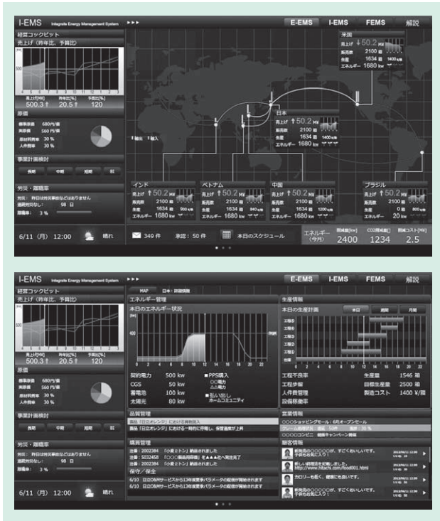
Fig. 7—Factory Management Cockpit Solution Screens. The screens show KPIs for each level from a global management perspective (top) down to a factory perspective (bottom), and also workplace information.
