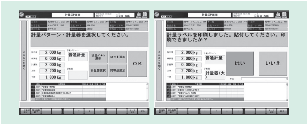
Fig. 3—SOP Screens. The screens show standard operation procedures (SOPs) displayed by Hitachi MES for process industries. Features include multilingual support and the ability to use text, images, video, and audio.
