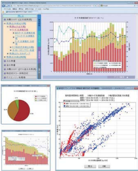
Web screen from energy management system for heating and cooling equipment
