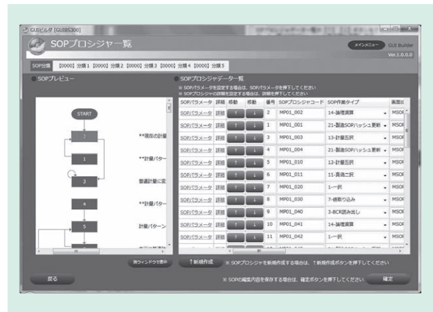
Fig. 5—Self-engineering Screen. The screens, text, and other information to be used (right) can be assigned to work procedures (left).
