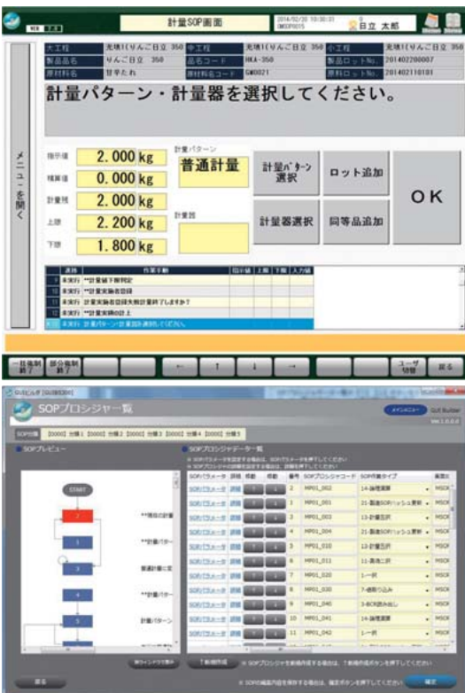
Screen from manufacturing execution system for process industries
