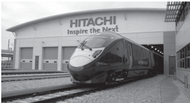
Fig. 1—Class 395 Rolling Stock. This Class 395 train is at the Ashford depot where Hitachi operates the maintenance services it has been contracted to supply.
