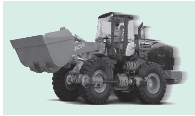
Fig. 4—Cutaway Diagram of ZW220HYB-5B Power Train. Despite incorporating the hybrid system, the ZW220HYB-5B has the same vehicle appearance and dimensions as the previous model.
