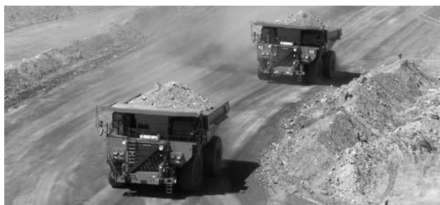
Demonstration project for autonomous haulage dump-trucks underway at a mine in Australia
