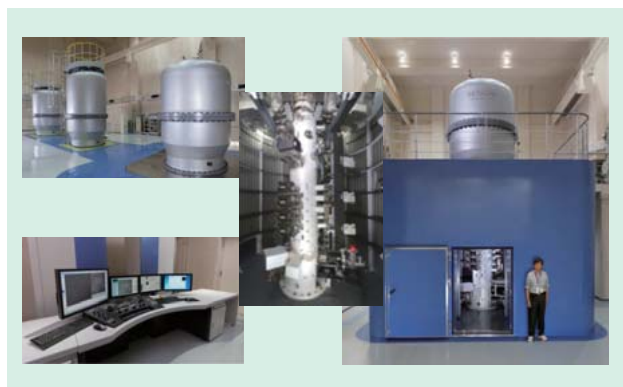
Fig. 11—Atomic-resolution Holography Electron Microscope. The photographs show the three large high-voltage tanks (top-left), the electron microscope operation console (bottom-left), the electron microscope itself (lens, specimen stage, detector, etc.) (center), and the electron microscope viewed from the front (right).
