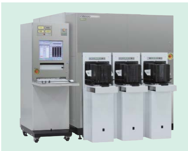
Fig. 2—CD-SEM for Use in Semiconductor Production. This is a photograph of the CG5000 high-resolution field emission beam critical dimension scanning electron microscope (FEB CD-SEM) (Hitachi High-Technologies Corporation). The CG5000 is used for the dimensional measurement of the patterns formed on semiconductor or other wafers.
