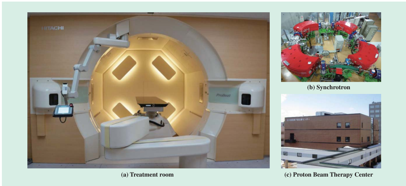
Fig. 1—Proton Beam Therapy System at Hokkaido University Hospital Proton Beam Therapy Center. (a) Treatment room equipped with rotating gantry. The irradiation field shaping mechanism (located under the table) enables the proton beam to be directed at the patient from any angle (360°). (b) The proton beam is accelerated by a synchrotron accelerator. (c) The Proton Beam Therapy Center is located next to Hokkaido University Hospital for easy access by patients.
