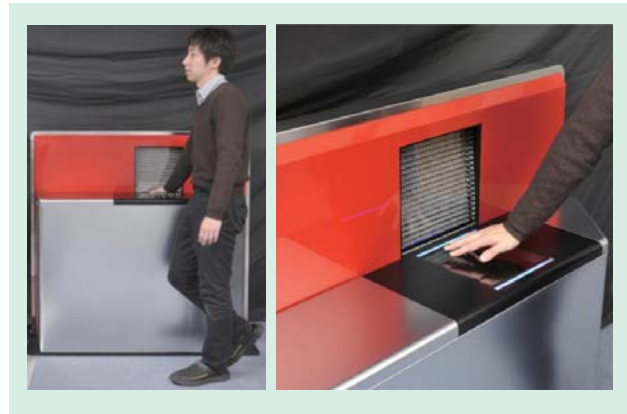
Fig. 4—Walkthrough-style Finger Vein Authentication Unit. The unobstructed access to the interface enables users to place their fingers on the reader and identify themselves as they walk past.
