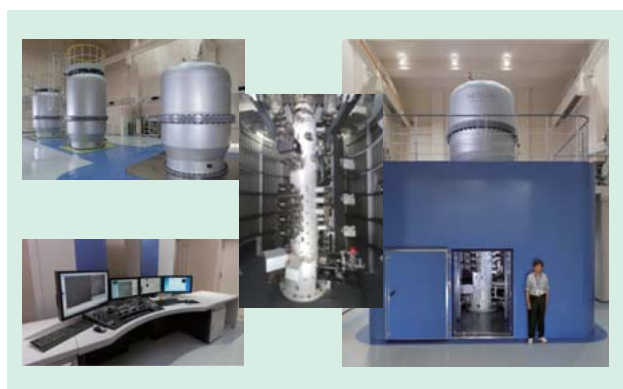
Fig. 11—Atomic-resolution Holography Electron Microscope. The photographs show the three large high-voltage tanks (top-left), the electron microscope operation console (bottom-left), the electron microscope itself (lens, specimen stage, detector, etc.) (center), and the electron microscope viewed from the front (right).
