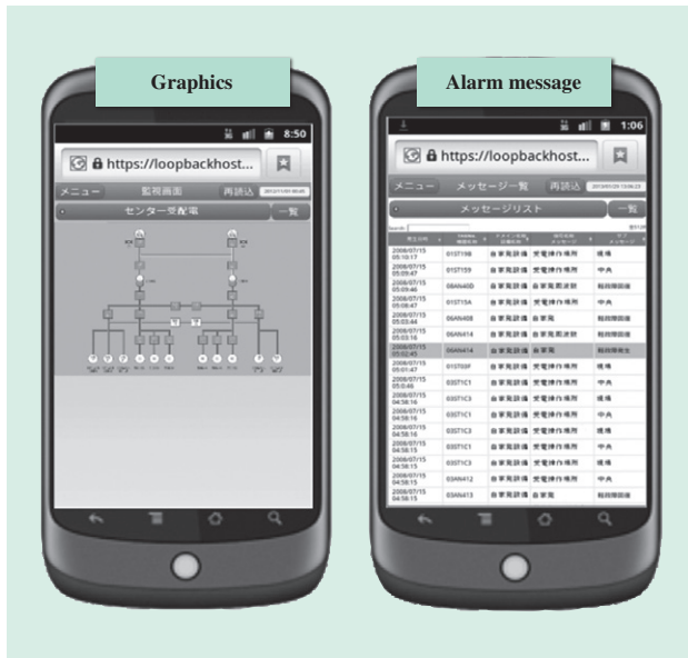
Fig. 6—Web Services Displayed on a Tablet. The web screens display the same graphics and alarm messages as the monitoring consoles at the Water Management Center. They also use familiar touchscreen operations such as pinch-out and swiping.
