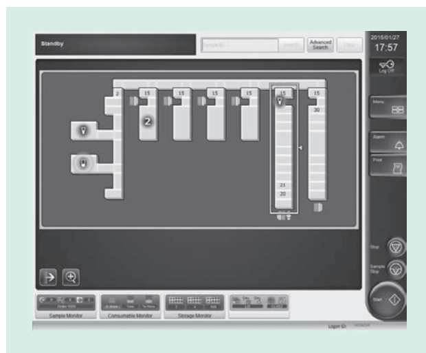
Fig. 5—The Laboratory Automation System Sample Monitor Screen. The screen is used to check the location and progress of specific samples.
