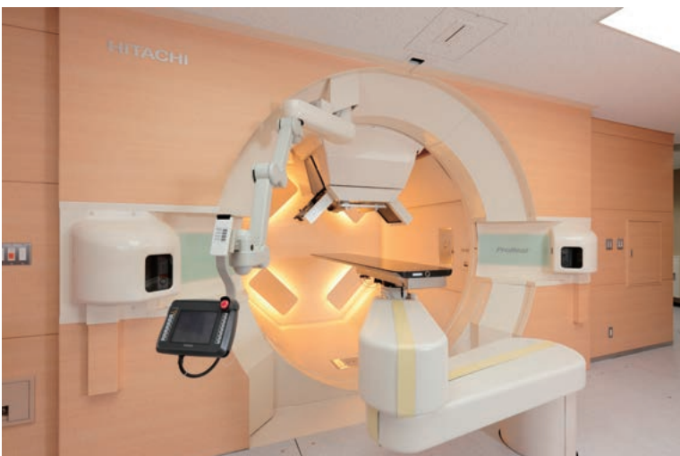
Therapy room for particle therapy system (Proton Beam Therapy Center, Hokkaido University Hospital)
