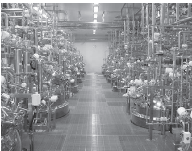
Fig. 1—High-volume Cell Culture System. This high-volume cell culture system (supplied by Hitachi, Ltd.) is used for the production of antibody drugs.
