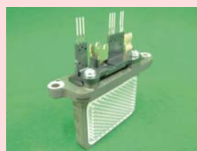
Power module with double-sided cooling
