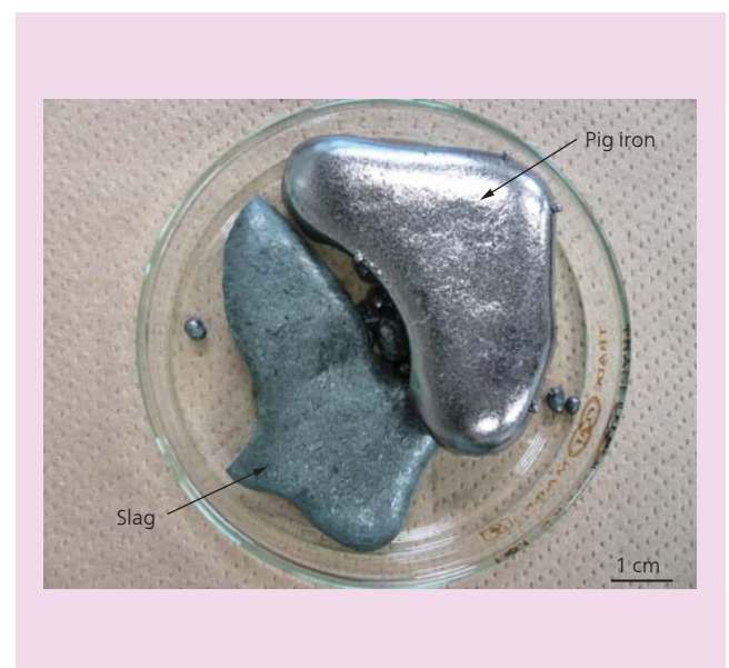
4 Material produced by carbothermal reduction of magnet sludge
