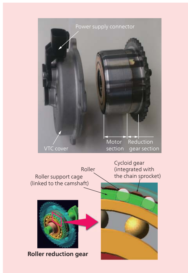
4 Integrated structure for a motorized VTC system with a DC brush motor and roller reduction gear (top) and roller reduction gear (bottom)
