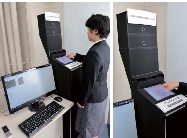
Prototype touch panel finger vein authentication system. The system provides enhanced convenience by performing authentication without the user’s awareness (but with their prior consent) by identifying their finger vein pattern as they use the touch panel, while at the same time taking a facial photograph.
