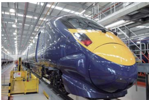
Maintenance depot for Class 395 high-speed trains in the UK. Work is proceeding on the use for predictive diagnosis of data collected from sensors fitted to the trains.
