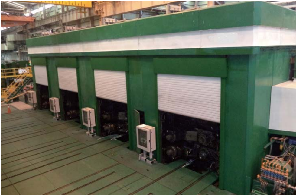
1 Aluminum tandem hot rolling mill for CSAC of Taiwan
