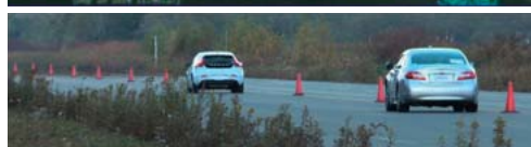
A demonstration of ACC using only small stereo cameras. Delicate control of the vehicle is needed to prevent the operation from feeling unnatural to people in the car.
