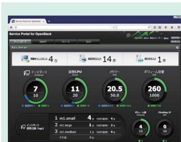
6 Example screen from Job Management Partner 1/Service Portal for OpenStack, a service portal for making OpenStack operation more efficient (left), and use of Job Management Partner 1 for centralized management of an entire multi-cloud environment (right)
