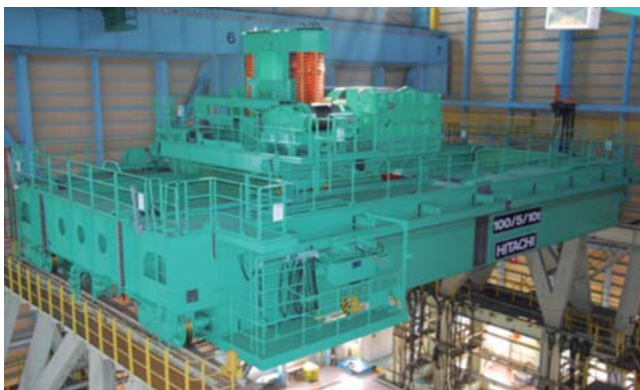
7 Factory testing of fuel removal and transportation crane for Unit 4 at Fukushima Daiichi Nuclear Power Station (the orange object is the spring shock absorber)
