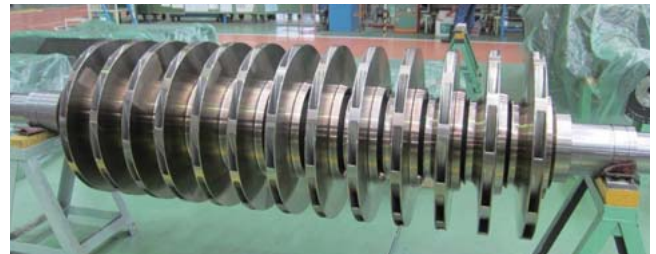
26 Compressor rotor with 13 impeller stages
