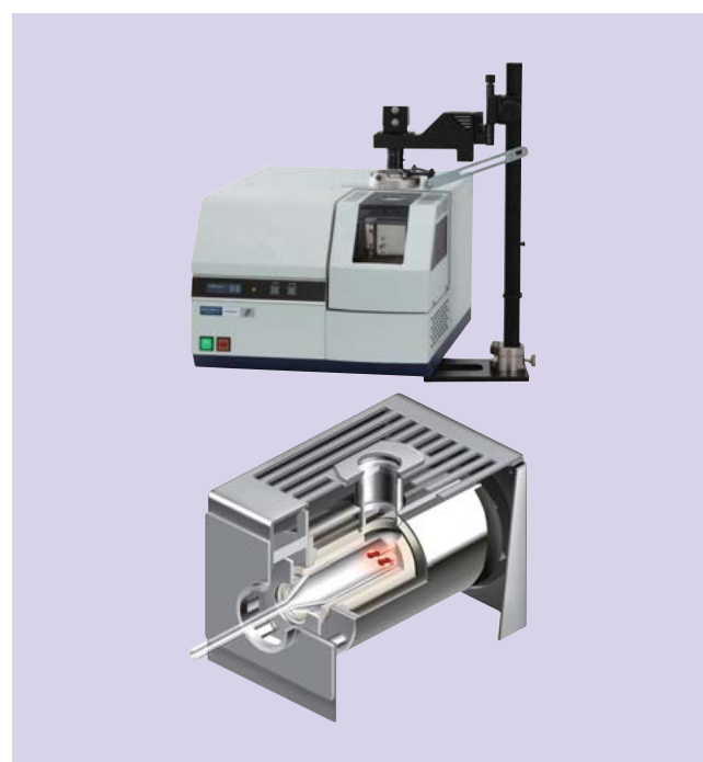
4 STA7200RV simultaneous thermogravimetric analyzer fitted with sample observation option (top) and heating furnace design with view port (bottom)
