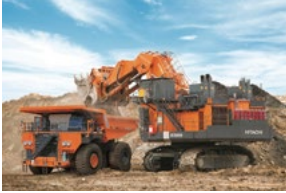
Hitachi Construction Machinery's ultralarge hydraulic excavator and dump truck for use in mining.
