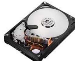
Hard disk drives (voice coil motor, spindle motor)
